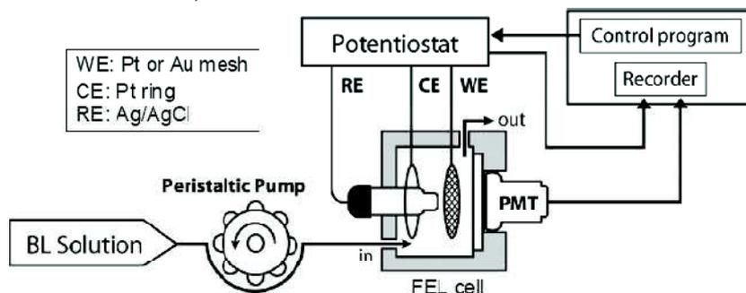
Figure 6. Schematic illustration of the flow-electrolysis luminescence (FEL) system
